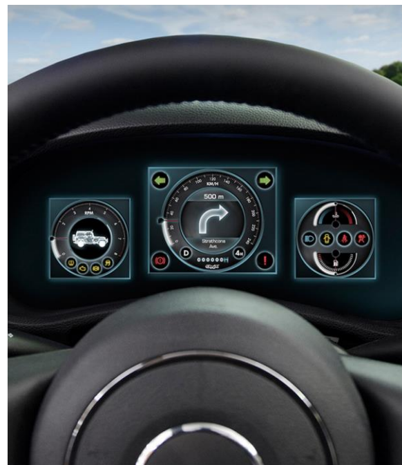
Figure 1. A digital instrument cluster showing information from components requiring different dependability levels
