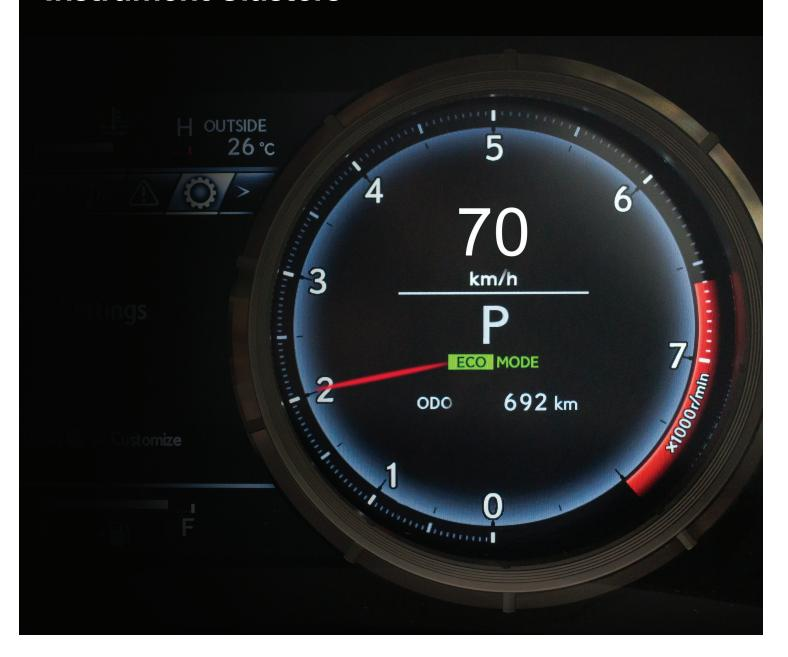
The QNX Platform for Instrument Clusters was created to help automakers and their Tier 1 suppliers respond to evolving challenges with the development of full digital instrument clusters. BlackBerry QNX ISO 26262 ASIL B pre-certified graphics stack, coupled with the ASIL D pre-certified RTOS and tool chain makes this innovative solution a powerful, customizable, and safety certified option for automakers.
